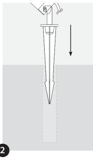
Gently push the spike into the ground to the desired depth. Don't put pressure on the head of the lamp.
